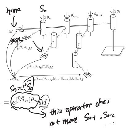
Apply screw motion to joint n:  $T_{sb}(0,\ldots,0,\theta_n)=e^{[0\bar{S}_n]\theta_n}$
