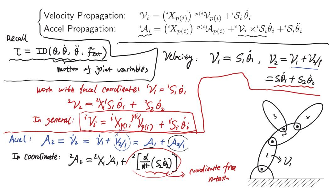
$$\frac{2}{2}\left[\frac{d}{dt}\left(S_{2}\dot{\theta}_{2}\right)\right] = \frac{d}{dt}\left({}^{2}S_{2}\dot{\theta}_{2}\right) + {}^{2}V_{2} \times {}^{2}S_{2}\dot{\theta}_{2} = {}^{2}S_{2}\dot{\theta}_{2} + {}^{2}V_{2} \times {}^{2}S_{2}\dot{\theta}_{2}$$
